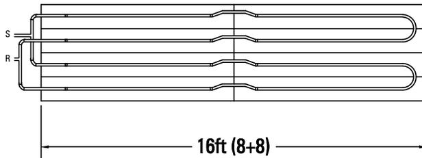
16 ft. x 2 pass/circuit = 32 ft./circuit @ 0.5GPM
