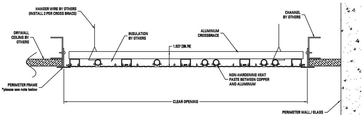
\*Perimeter frame by others. Note that SIGMA supplied frames DO NOT span from Wall to Wall
