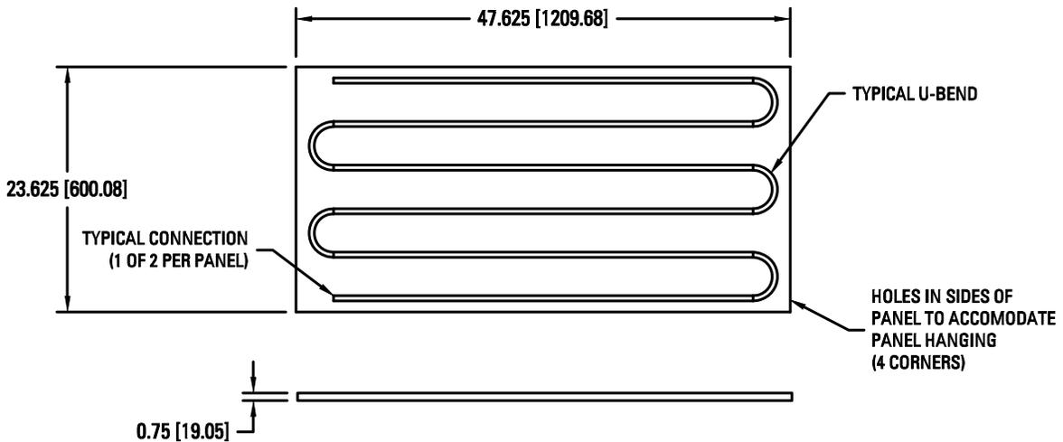
Note: 6 pass modular panels are shown on this page. Panel dimensions for 4 pass and 5 pass are the same as 6 pass.
