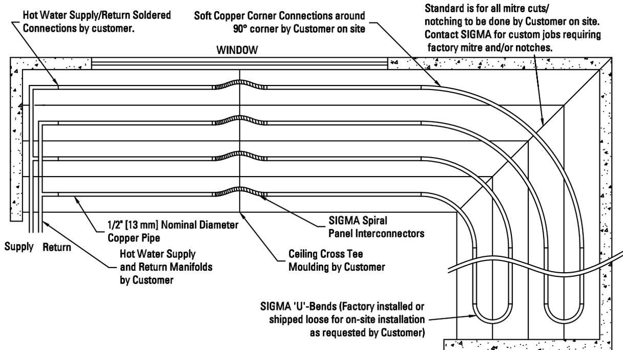
Parallel flow in even pass panels reduce pressure drop for long zones. SIGMA designs for 21 kPa (7 ft. H<sub>2</sub>O) maximum pressure drop, unless otherwise noted by customer.
